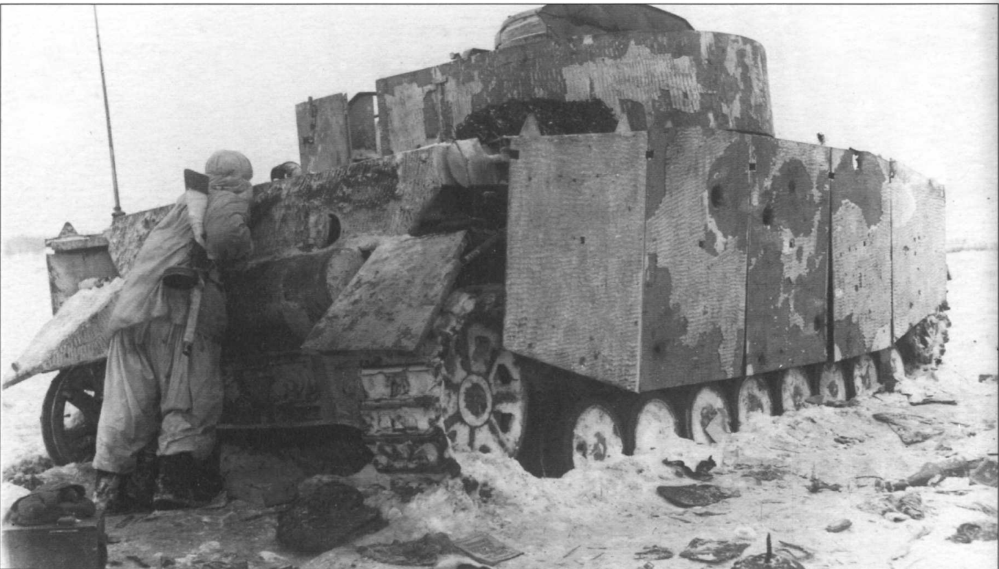
A grenadier takes cover behind a knocked out late variant PzKpfw IV during winter operations in 1944. It is evident from the number of shell holes in the tank's side skirts that it has been embroiled in a heavy contact with the enemy. The vehicle has probably had an internal fire as much of the Zimmerit and whitewash paint can be seen burnt off.
