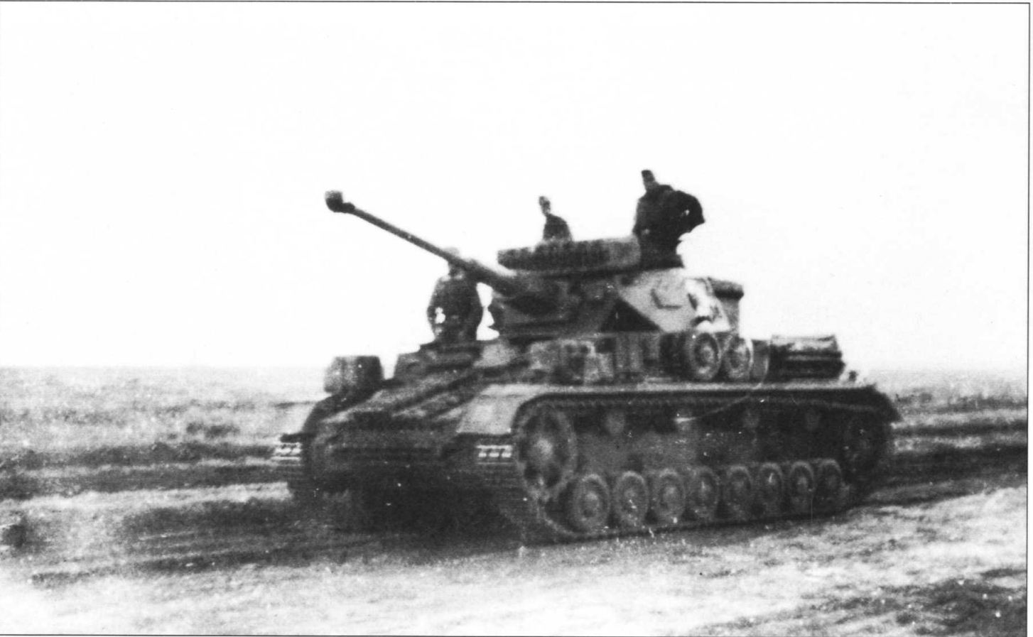
A PzKpfw IV moves hastily along a dusty road somewhere in southern Russia in the summer of 1943. Note the rack fitted with jerry cans on the turret roof, indicating the vehicle is in for a long road march.
