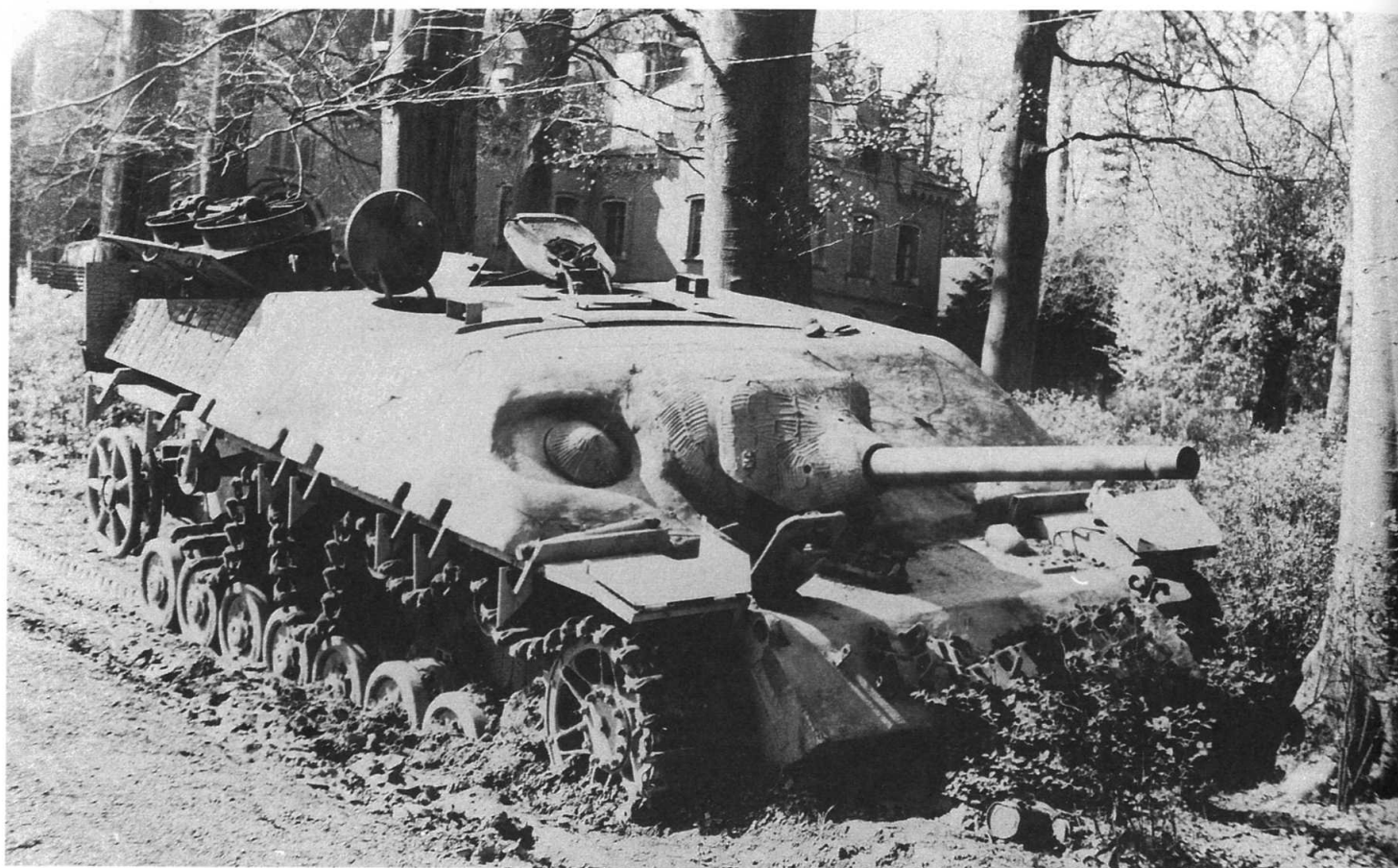
Another abandoned Jagdpanzer IV armed with the PaK 39 L/48. Note the engine doors at the rear of the vehicle are open showing the fans for the powerful Maybach HL120 TRM engine.
