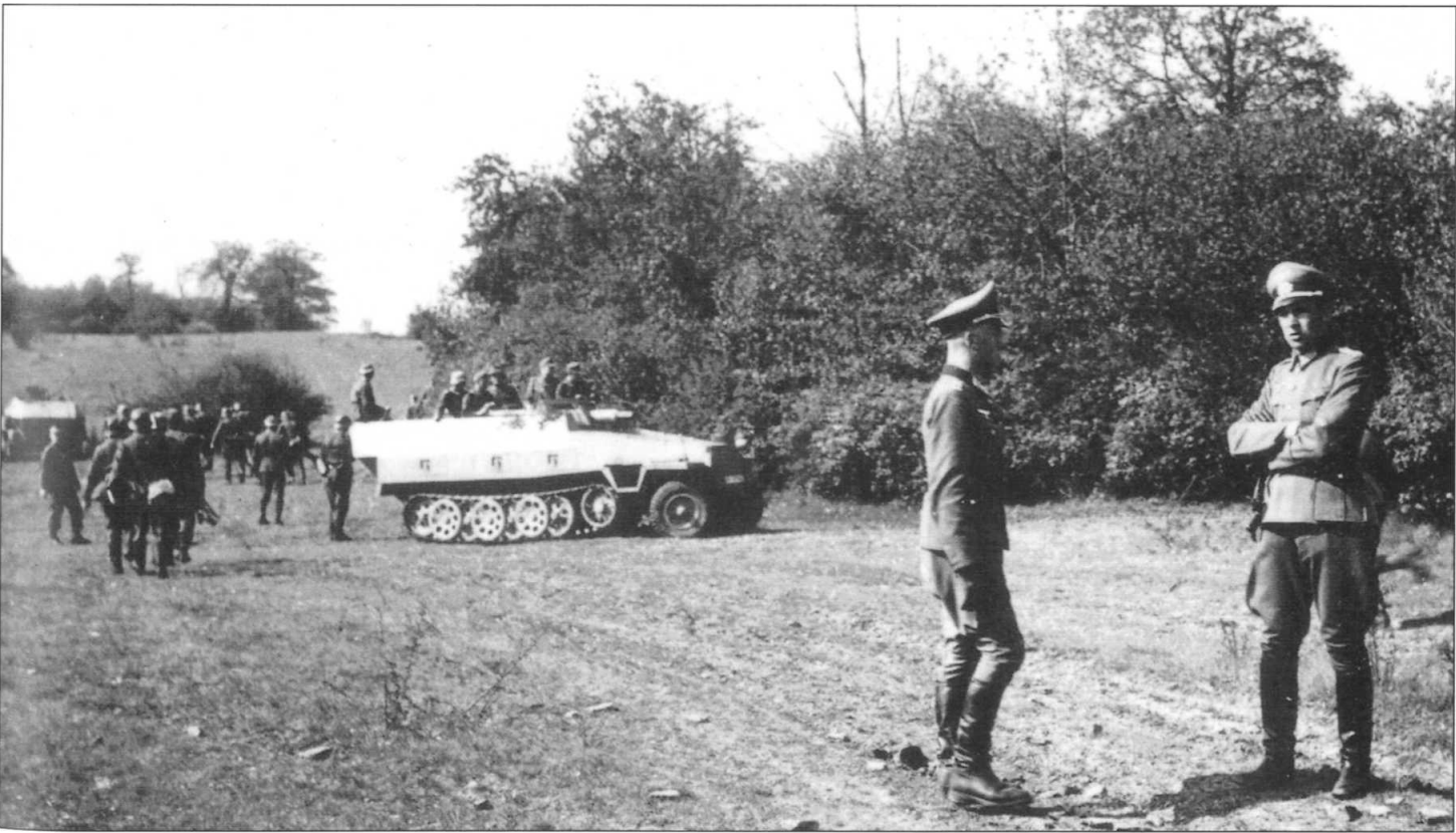
Two officers confer with each other whilst in the background an SdKfz 251/9 armed with the deadly short barreled 7.5cm KwK 37 L/24 is directed towards some trees. Dismounted Panzergrenadiers can be seen on foot following another SdKfz 251 through a hedgerow. Panzergrenadiers were the motorized infantry and generally travelled by motor vehicle than on foot. These troops were always moved into the thick of battle and provided armour with valuable support. [Michael Cremin]
