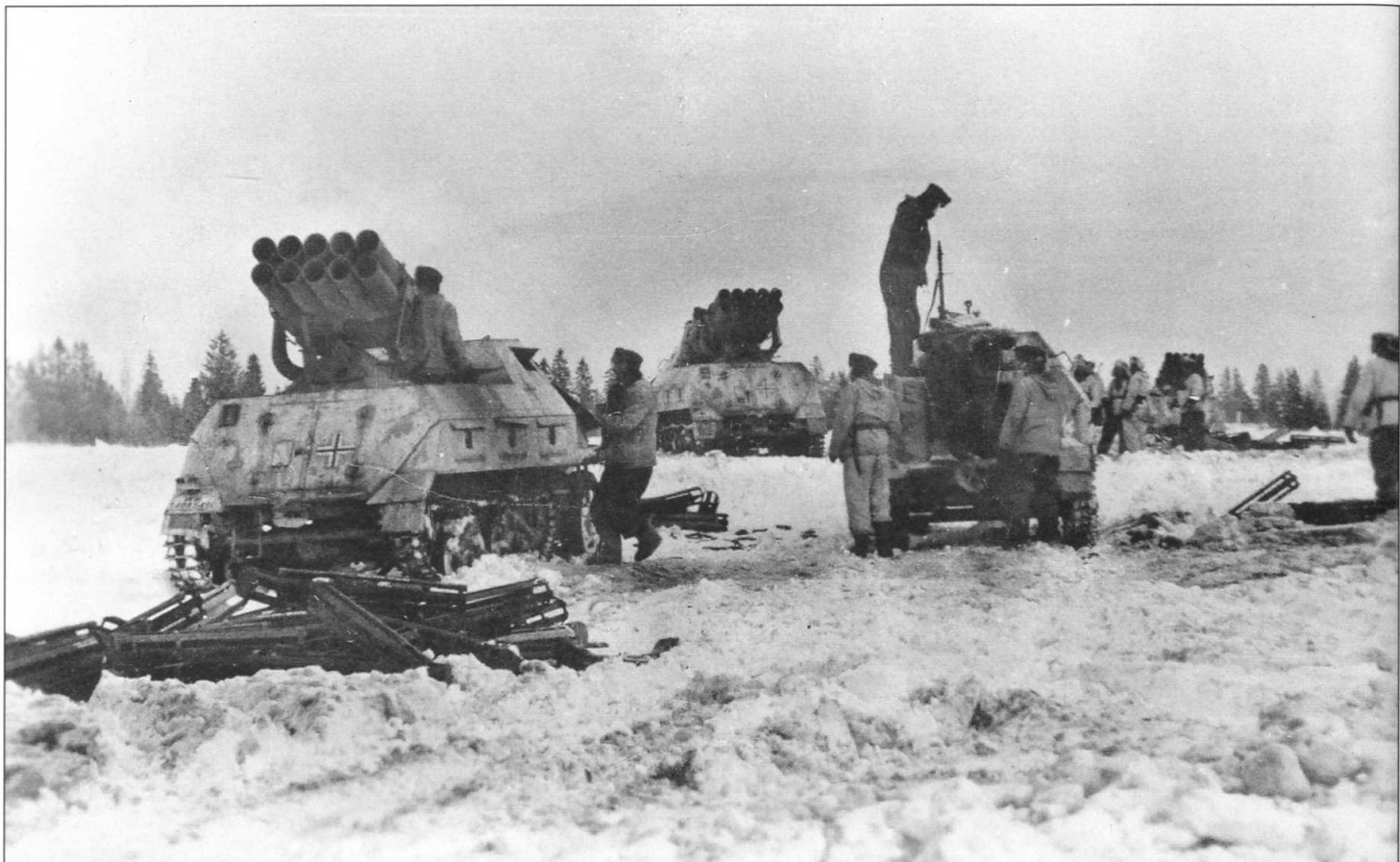
A number of Panzerwerfer and a munitions vehicle can be seen during a lull in the fighting in 1944. The vehicles are preparing for a firing mission during defensive operations in the east. These multi-barrelled rocket launchers could fire simultaneously 10 15cm rockets, and cause extensive damage to the enemy front lines.
