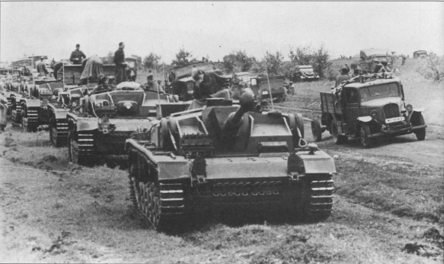
An impressive photograph showing a StuG III leading an armoured column. Because the StuG III was constantly in great demand in Russia Hitler ordered that the assault gun be up-gunned and up-armoured with a longer more potent 7.5cm gun. This more powerful assault gun went into production in mid-1942. The Ausf F variant mounted a 7.5cm StuK 40 L/43 gun. The following year the final StuG variant, the Ausf G, entered service with the Panzerwaffe .
