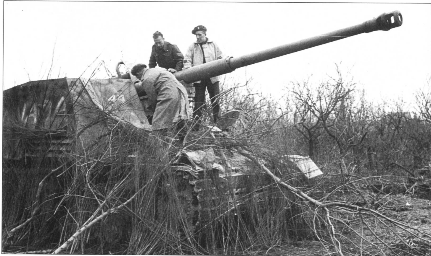
Polish soldiers examine a captured Nashorn in early 1945. Branches from trees have been applied to the side of the vehicle in order to try and conceal it from enemy observation. The high profile of the Nashorn made it hard to conceal, but its long-range gun enabled it to fight at more extreme ranges than other tank destroyers.
