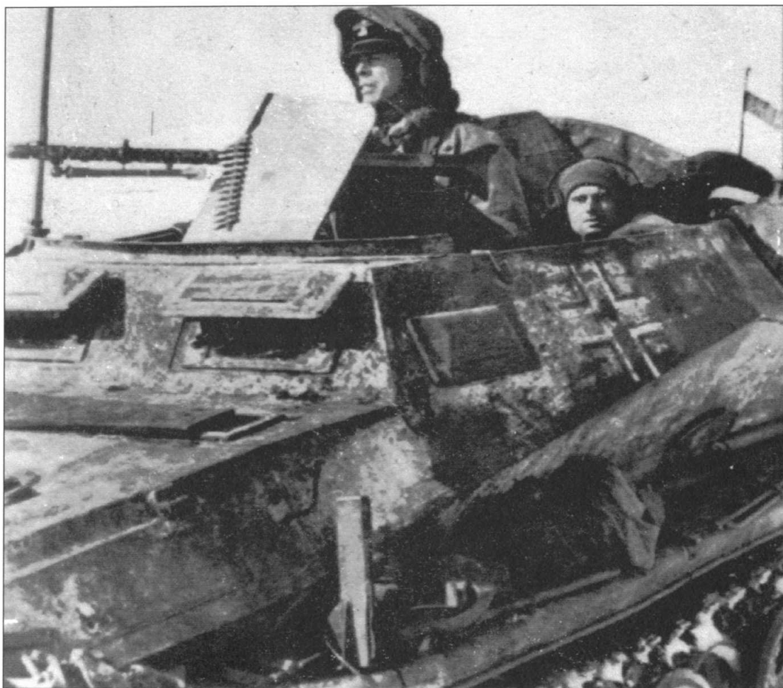
Two crewmembers can be seen inside an SdKfz 250 during operations in Poland in late 1944. This whitewashed vehicle is armed with an MG34 machine gun with splinter shield.
