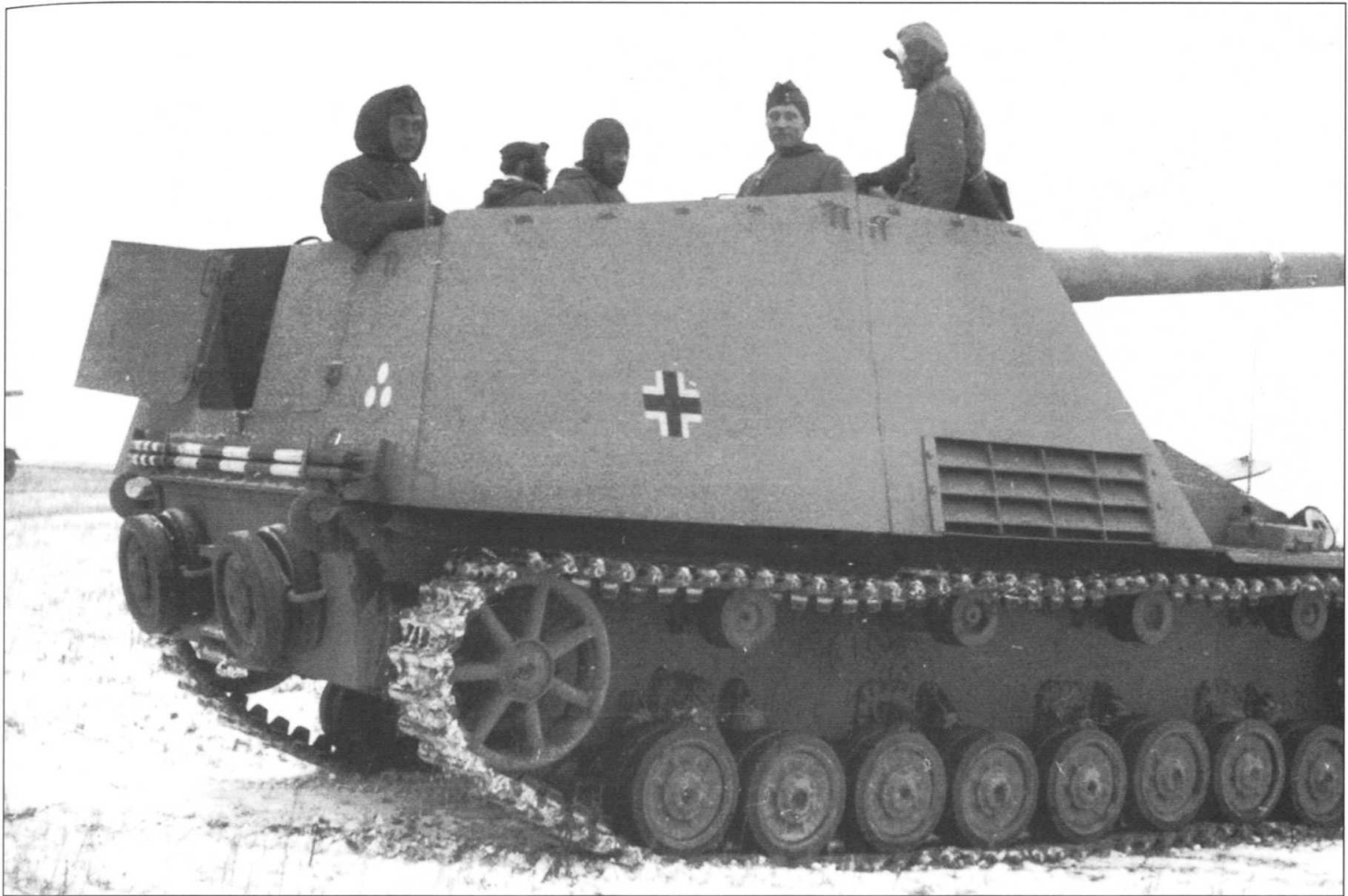
An SS crew wearing winter reversibles grey side out can be seen in the fighting compartment of a stationary Hummel. The Hummel mounted a standard 15cm heavy field howitzer in a lightly armoured fighting compartment built on the chassis of a PzKpfw III/IV. This heavy self-propelled gun carried eighteen 15cm rounds, but was a potent weapon against Soviet armour.
