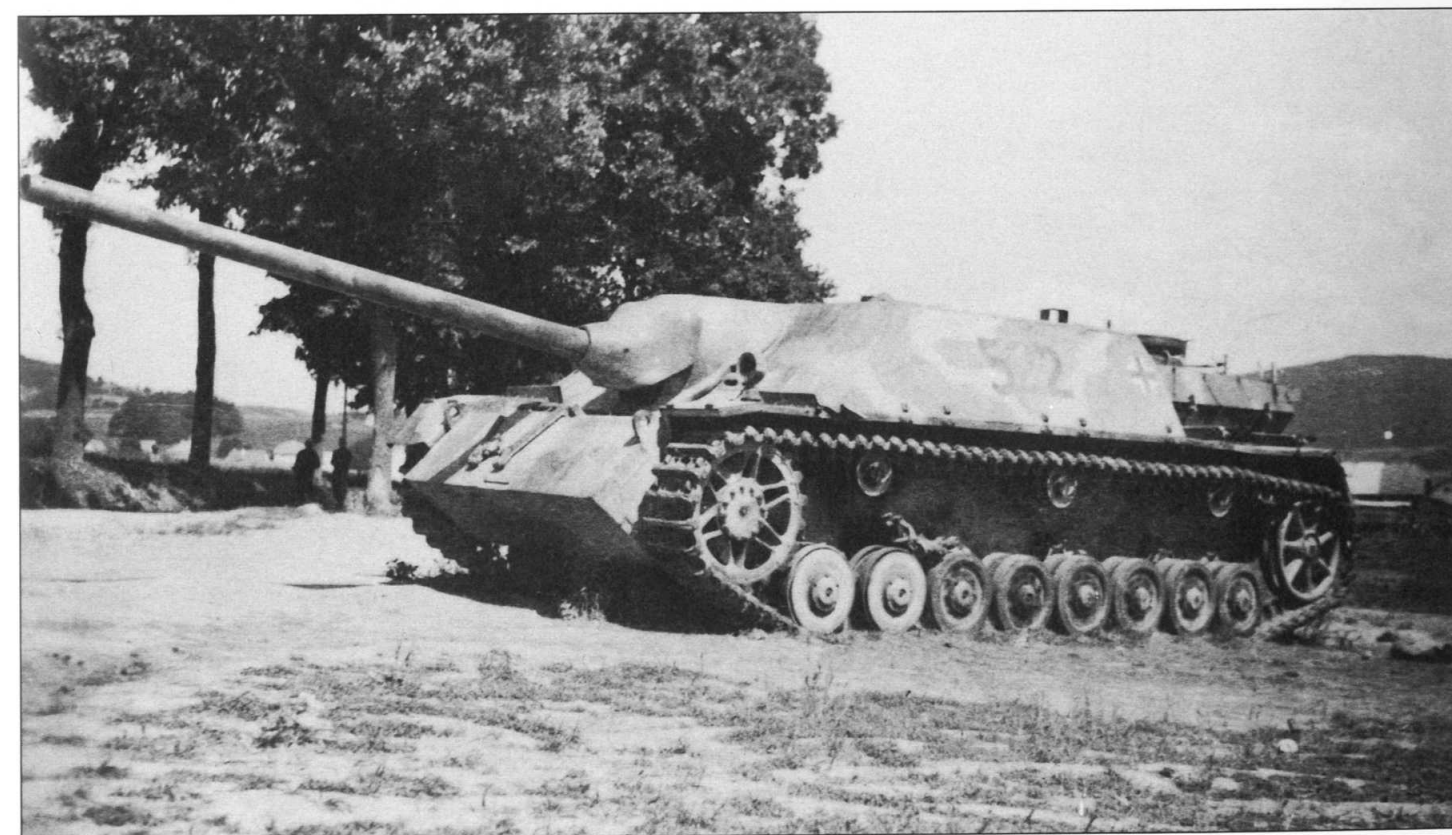
Three photographs showing abandoned Jagdpanzer IV's. With a drastic need for new armoured fighting vehicles, more second generation tank destroyers were built. One such vehicle that came off the production line in 1944 was the Jagdpanzer IV. This vehicle, built on the chassis of a PzKpfw IV, weighed 28.5 tons and was nicknamed 'Guderian's duck'. The vehicle was equal to any enemy tanks thanks to its potent 7.5cm gun. The Jagdpanzer saw extensive service in the east and with its reliability and well-sloped thick frontal armour it became a highly efficient fighting vehicle, if only for a short period of time.
