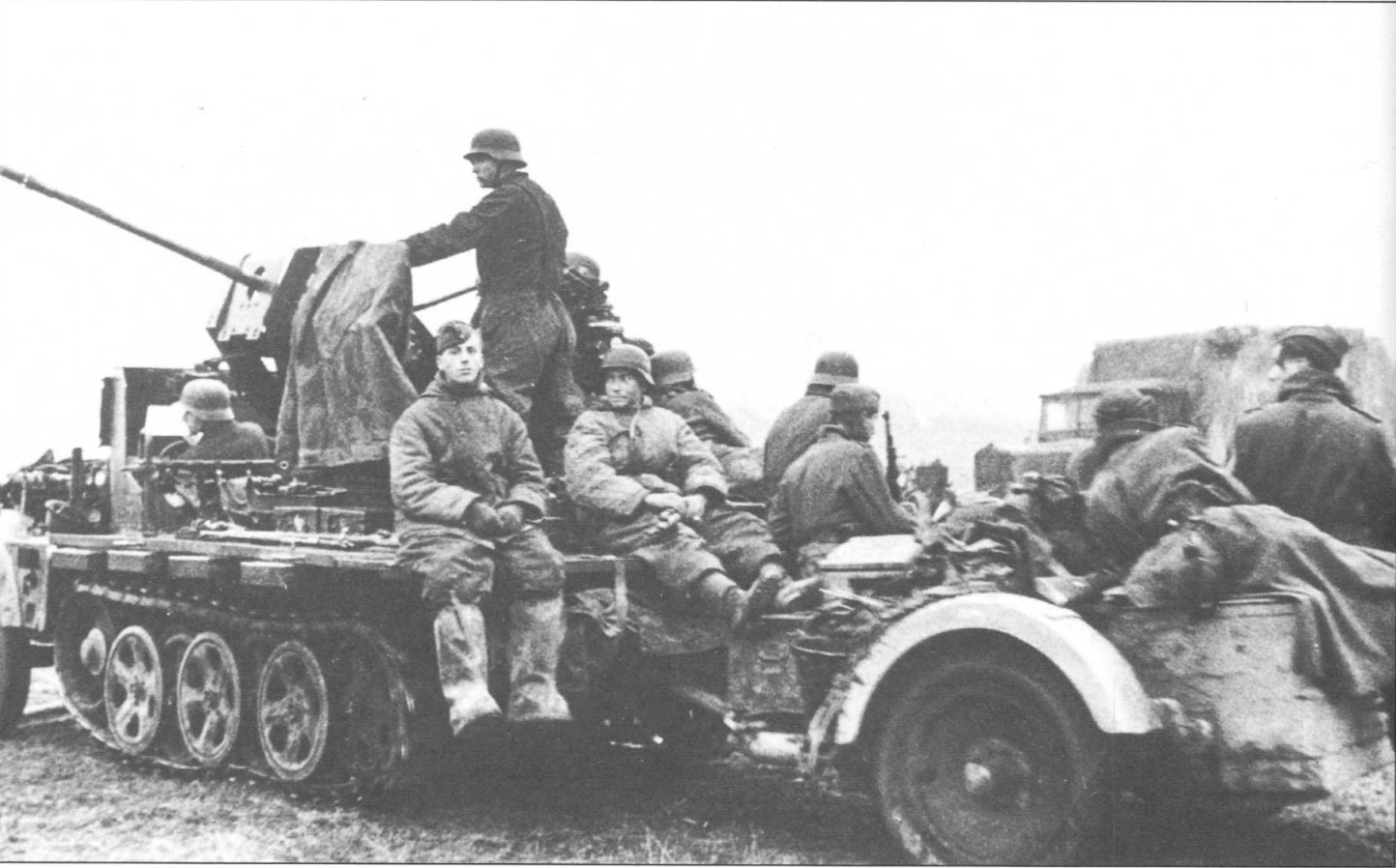
Moving steadily west grenadiers hitch a lift onboard an artillery tractor. Mounted on the back of the SdKfz 10/4 halftrack is a 2cm flak gun. The vehicle is towing an Sd.Ah.51 ammunition trailer.
