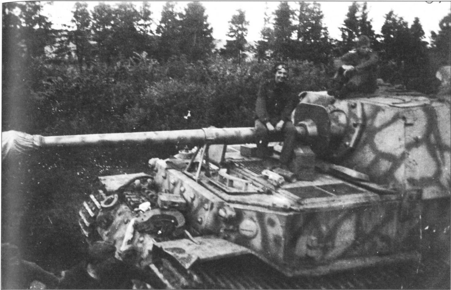
An Elefant tank destroyer stationary on a road with its crew during operations in the later stages of the war. The vehicle carries a very interesting camouflage pattern of dark yellow with red brown and olive green wavy lines.
