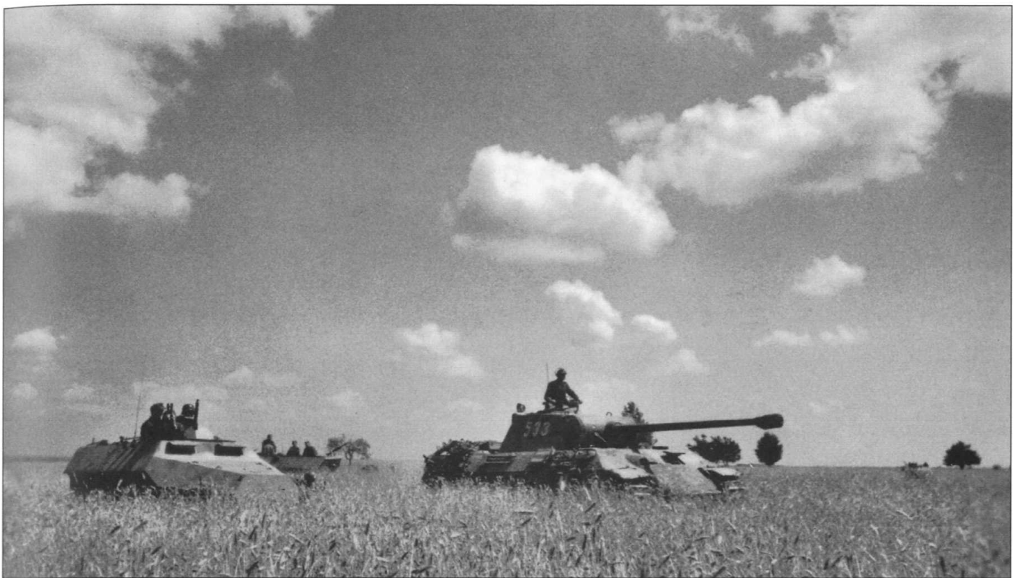
Armoured vehicles consisting of two stationary SdKfz 251 halftracks and a PzKpfw V Panther halted in a wheat field. The Panther first appeared at Kursk in July 1943, making a rather inauspicious operational debut. By 1944, however, following a number of successful improvements, it dominated the battlefield. [Michael Cremin]
