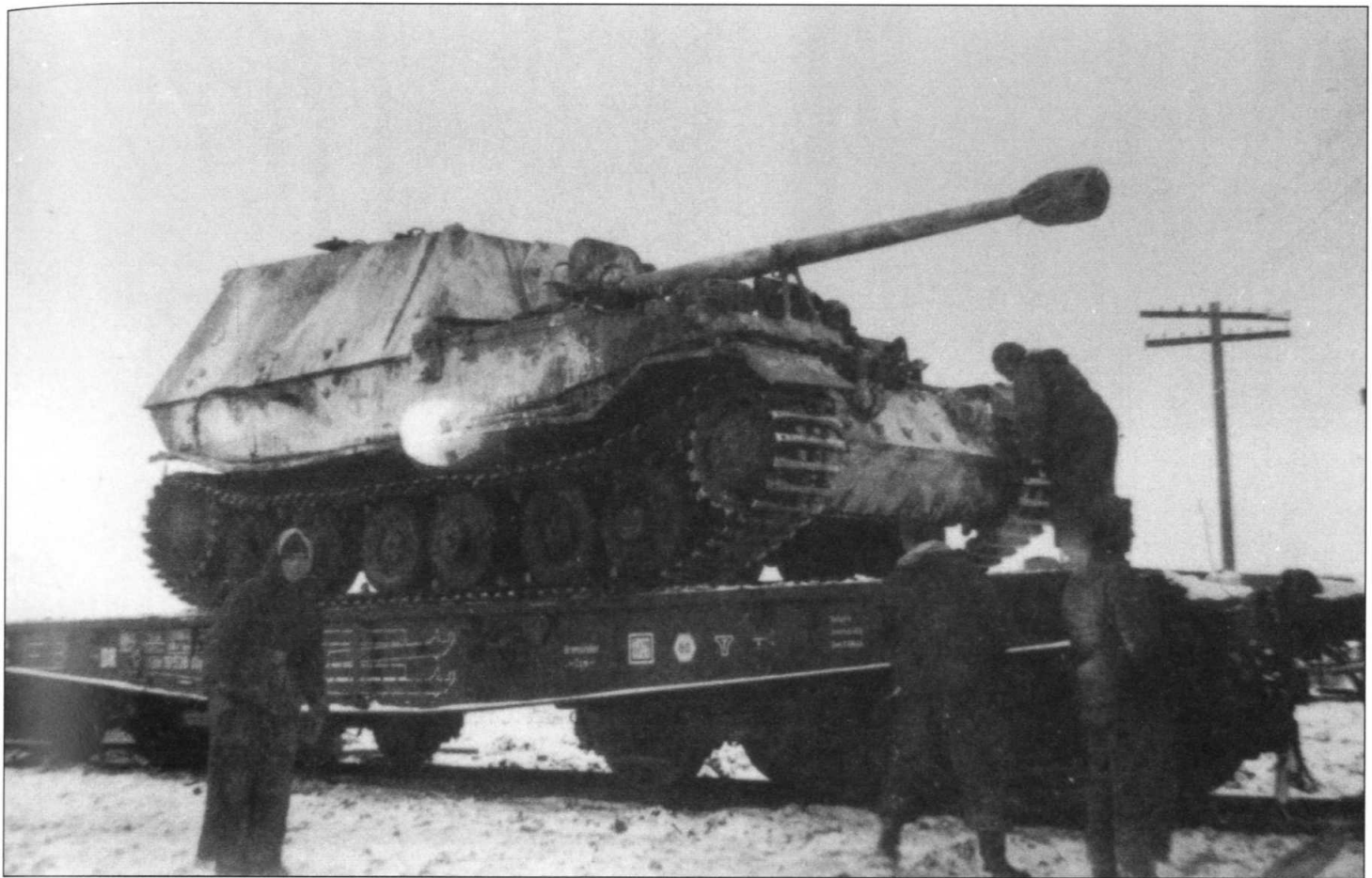
Two photographs showing Panzerjäger Tiger or Ferdinand Elefant tank destroyers that have been chocked and secured ready for their journey by rail. Due to their sheer size and weight, no more than six of these vehicles were permitted to be loaded on one train. These were interspersed with two flatcars to avoid overloading of the train, and also to prevent overloading of the bridges.
