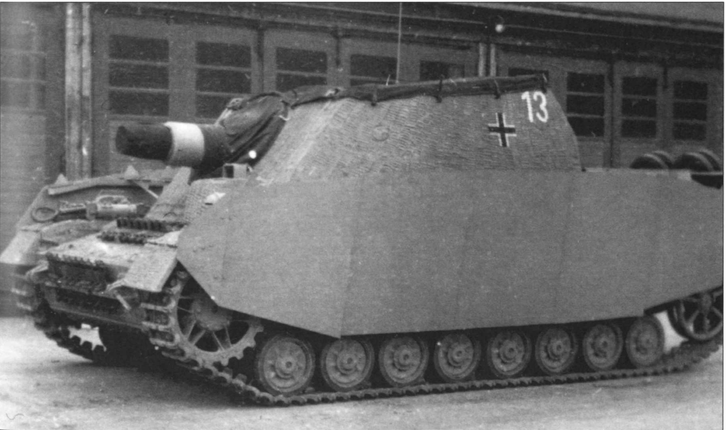
Here a Sturmpanzer IV Brummbär is parked ready for deployment in the summer of 1944. The Brummbär or 'grizzly bear' as it was nicknamed, mounted the powerful sIG 15cm gun. In early August 1944 10 Sturmpanzers were transferred to Army Group Centre to assist in suppressing the Warsaw uprising.
