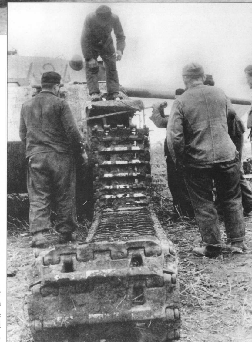
A Panther crew is preparing to change tracks for cross-country combat operations. The Panther tracks were fitted with chevroned cleats intended to increase traction and reduce slipping on icy conditions and on hard surfaces such as concrete and cobblestones.
