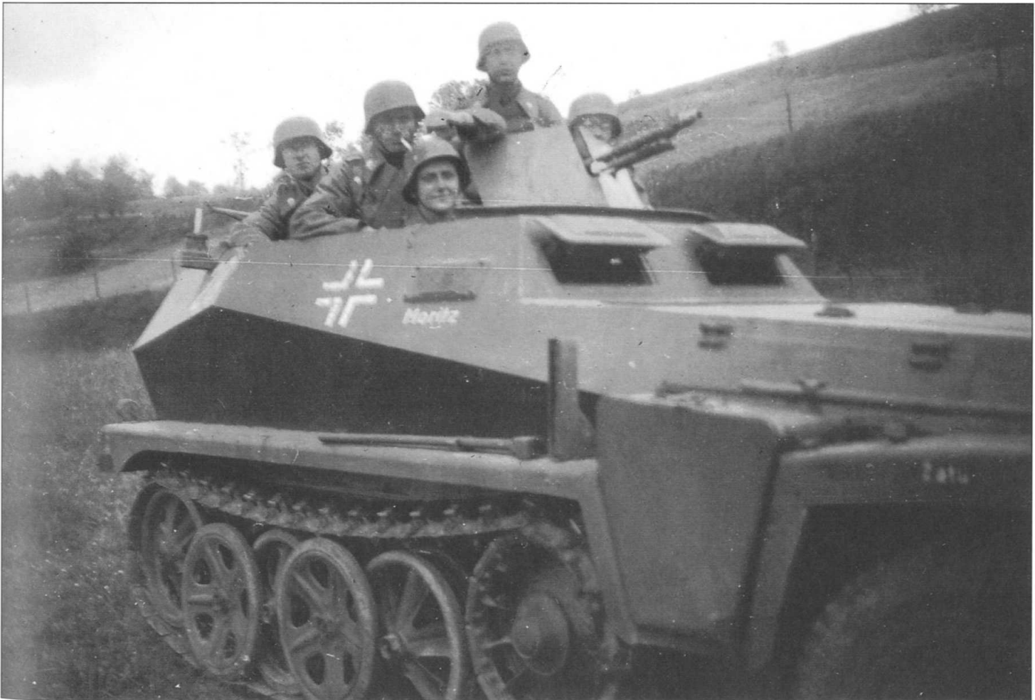
The crew of an SdKfz 250/1 passes through a field and are all captured on film facing the camera. The SdKfz 250 was designed purely to provide armoured reconnaissance troops in the Panzer and Panzergrenadier divisions with better off-road performance than the SdKfz 222. These light armoured personnel carriers normally carried six troops and were armed with either an MG34 or MG42 machine gun, which can be seen in this photograph with splinter shield
