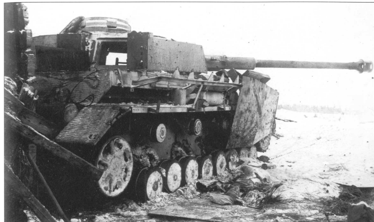
A destroyed PzKpfw IV on the Eastern Front during the winter of 1944/45. The vehicle appears to have received a direct hit and as a consequence of the shell's impact it has blown off most of the side-skirts. A thick coating of Zimmerit is evident over the chassis and turret.
