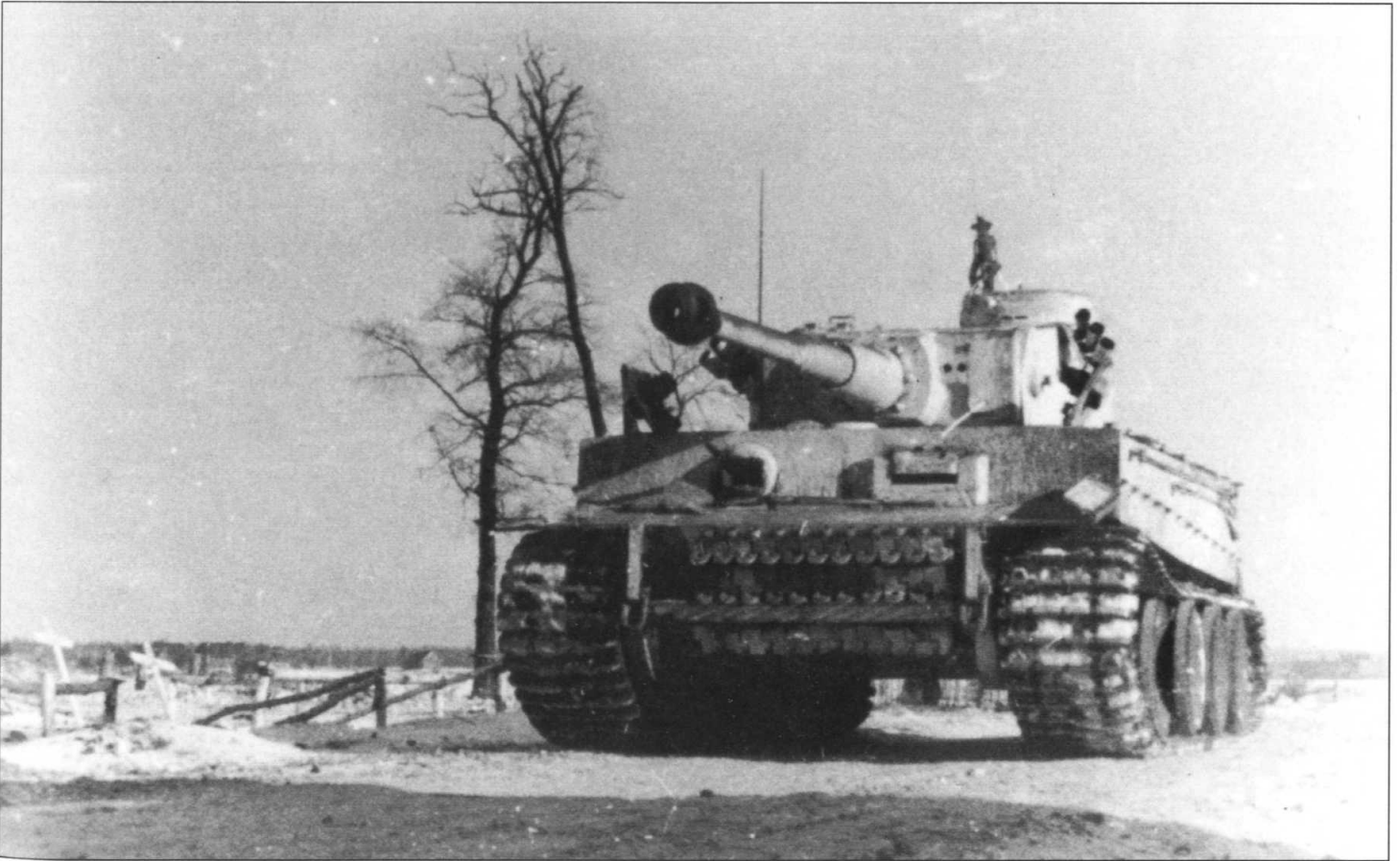
A Tiger I moves along a snow-covered road bound for the front line. This vehicle is well camouflaged with a good overall application of winter whitewash paint. Track links have been bolted to the front of the tank for additional armoured protection.
