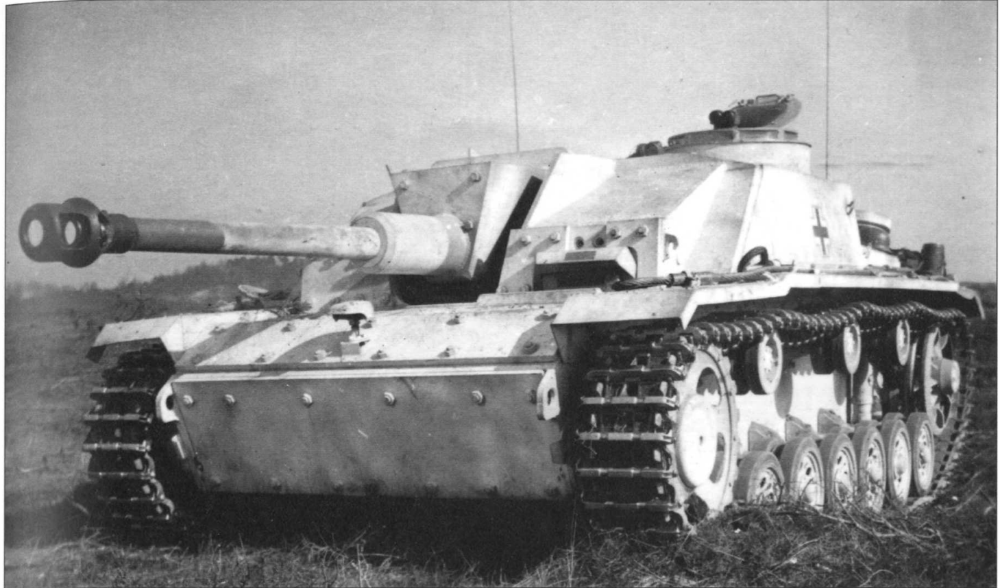
A StuG III Ausf G in a field with a full covering of winter whitewash paint. By 1943 the StuG III had become an extremely common assault gun in the Panzerwaffe on the Eastern Front. Its low profile and mechanical reliability saw its employment grow on the battlefield.
