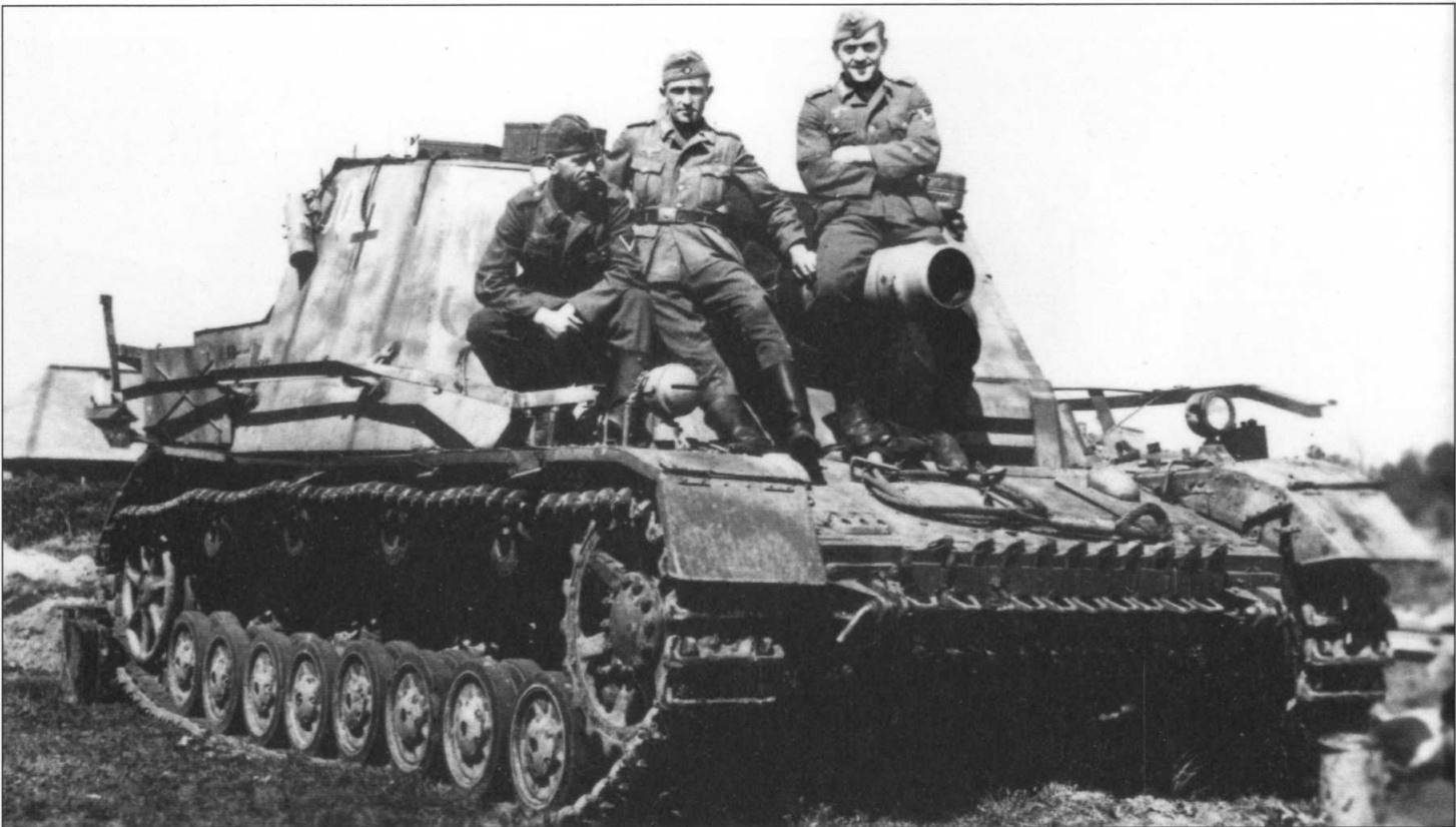
Members of the crew of a Sturmpanzer Brummbär sit proudly atop their vehicle. This was a powerful infantry support weapon developed in consequence of experiences fighting in Stalingrad. Armed with a powerful 15cm StuH 43 L/12 gun, 306 examples were built.
