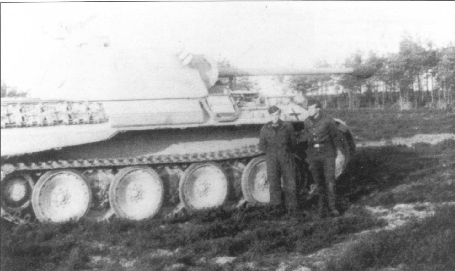
Two crewman stand beside their Panther during a training exercise. This variant mounts six smoke candle dischargers, three on each side of the turret. These were discontinued in production during June 1943. However, some Panthers still carried them for a number of months until they were finally removed.
