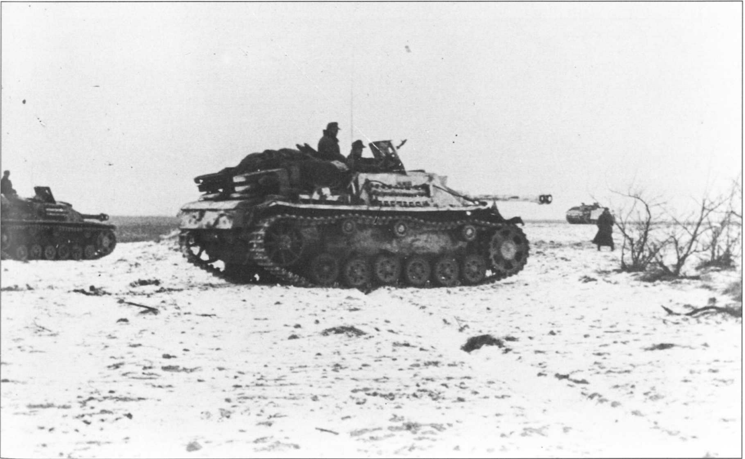
Three StuG III Ausf G take up positions on the open steppe during winter operations in 1944. Note that two of the assault guns have their side-skirts missing, these often being torn off during combat. The farthest assault gun appears to retain all its skirting.
