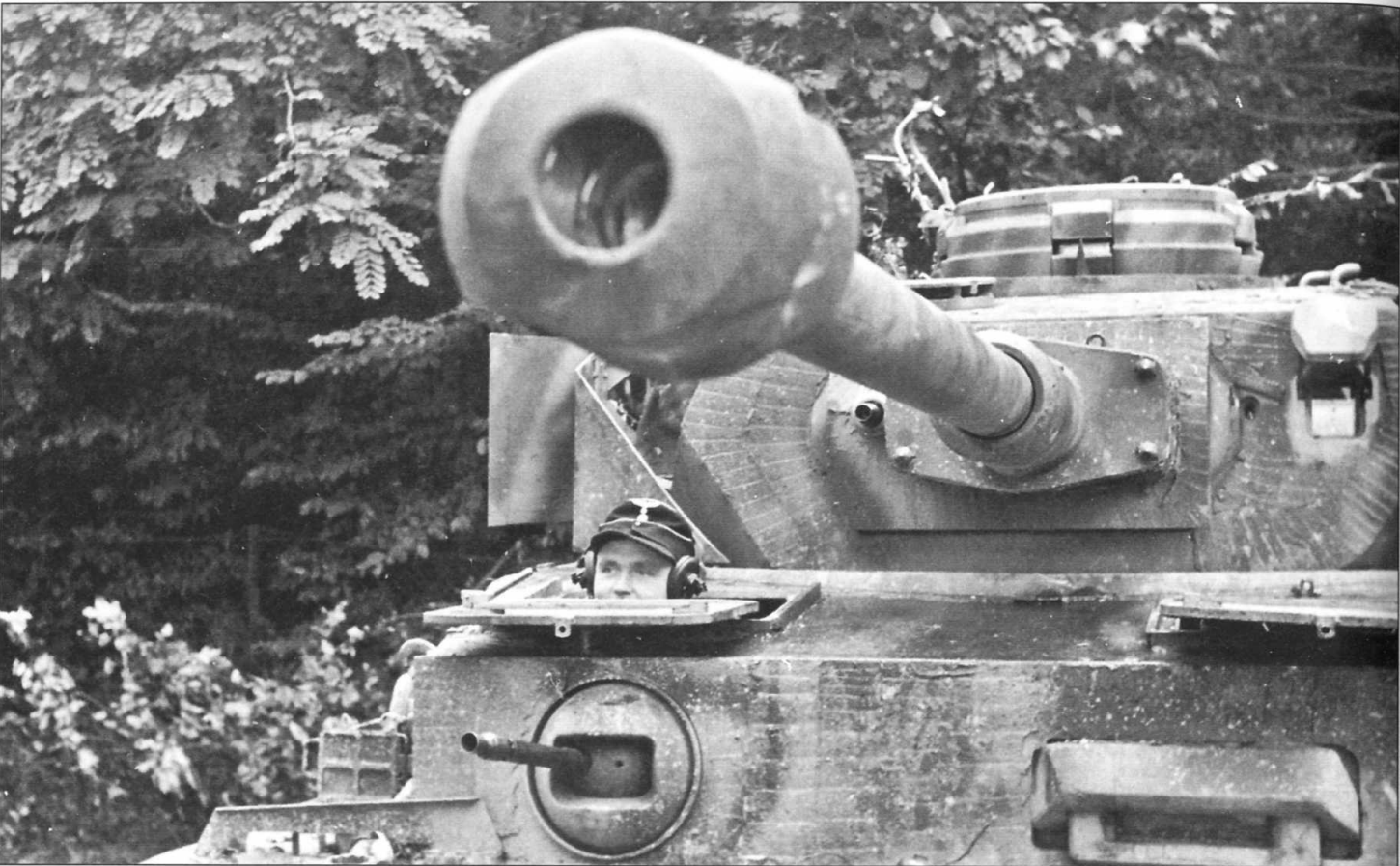
A crewman poses for the camera in his PzKpfw IV Ausf G command tank. Note the Zimmerit anti-magnetic mine paste on the superstructure. The vehicle has received a coating of dark yellow over sprayed with patches of olive-green and red-brown.
