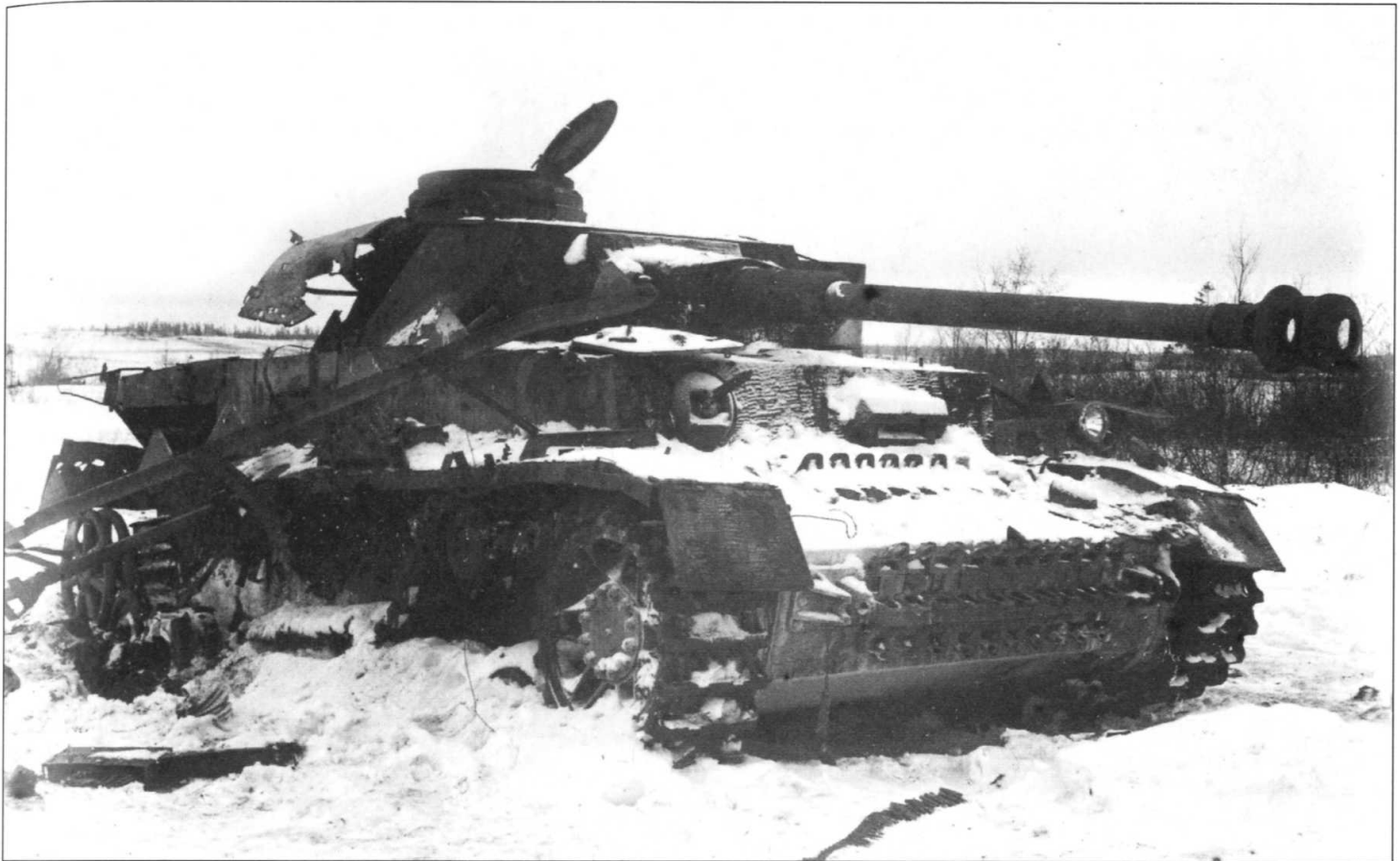
A knocked out PzKpfw IV in the snow. This tank has more than likely been hit by an anti-tank shell to the side of the vehicle and as a result the impact has blown part of the track off. Other damage is also visible along the side of the tank.
