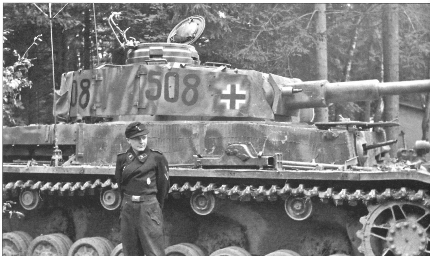
An interesting photograph showing a crewman posing for the camera in front of his PzKpfw IV Ausf G command tank in the summer of 1944. Note the coating of Zimmerit plaster coating on the vehicle, and the spaced armour plates around the turret, plus the star antenna.
