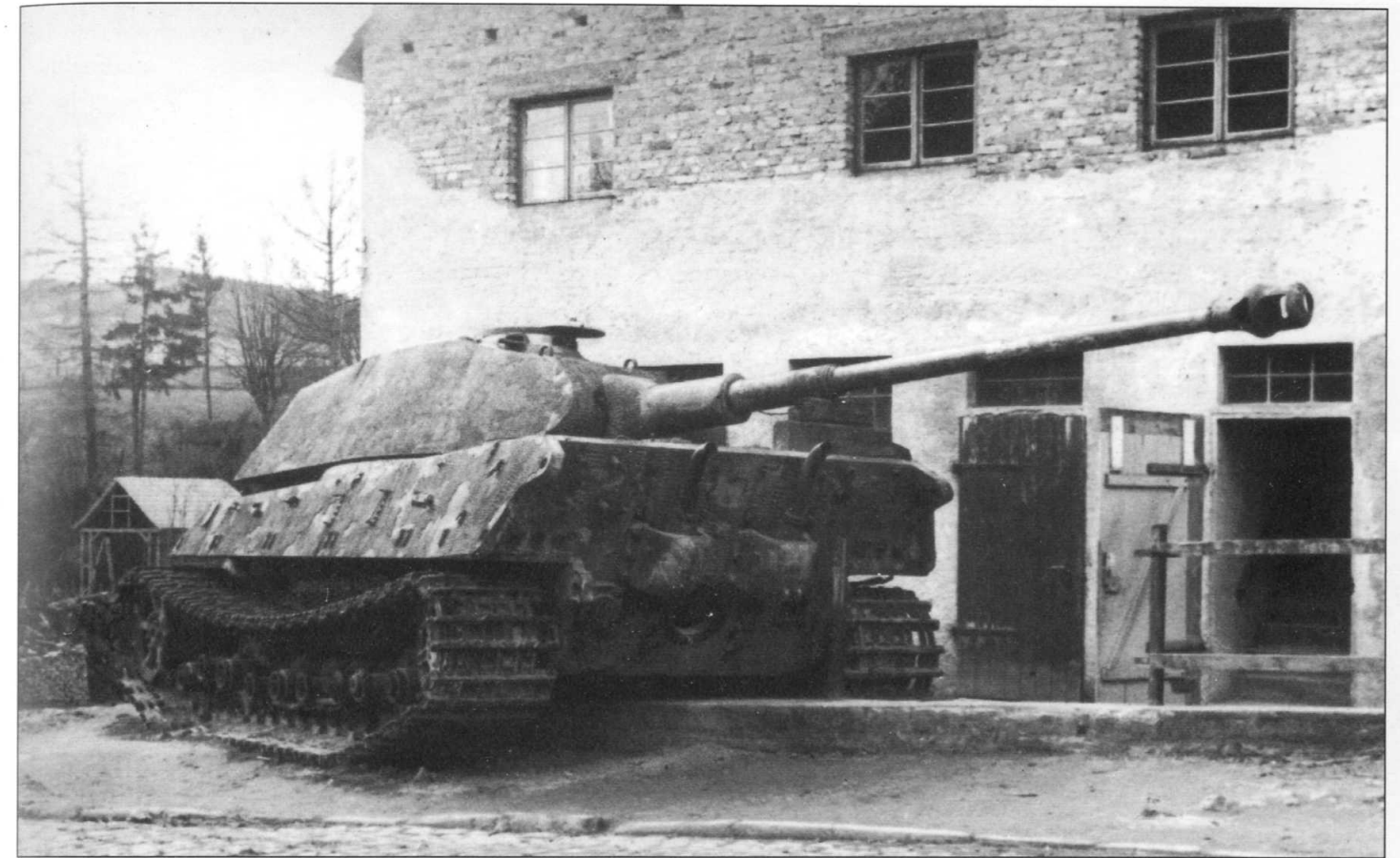
An abandoned Tiger II in the spring of 1945. This massive tank was introduced in the ranks of the Panzerwaffe in early 1944. It had a powerful 8.8cm KwK 43 gun with a barrel over 20ft in length, whilst the rounds weighed some 20kgs.
