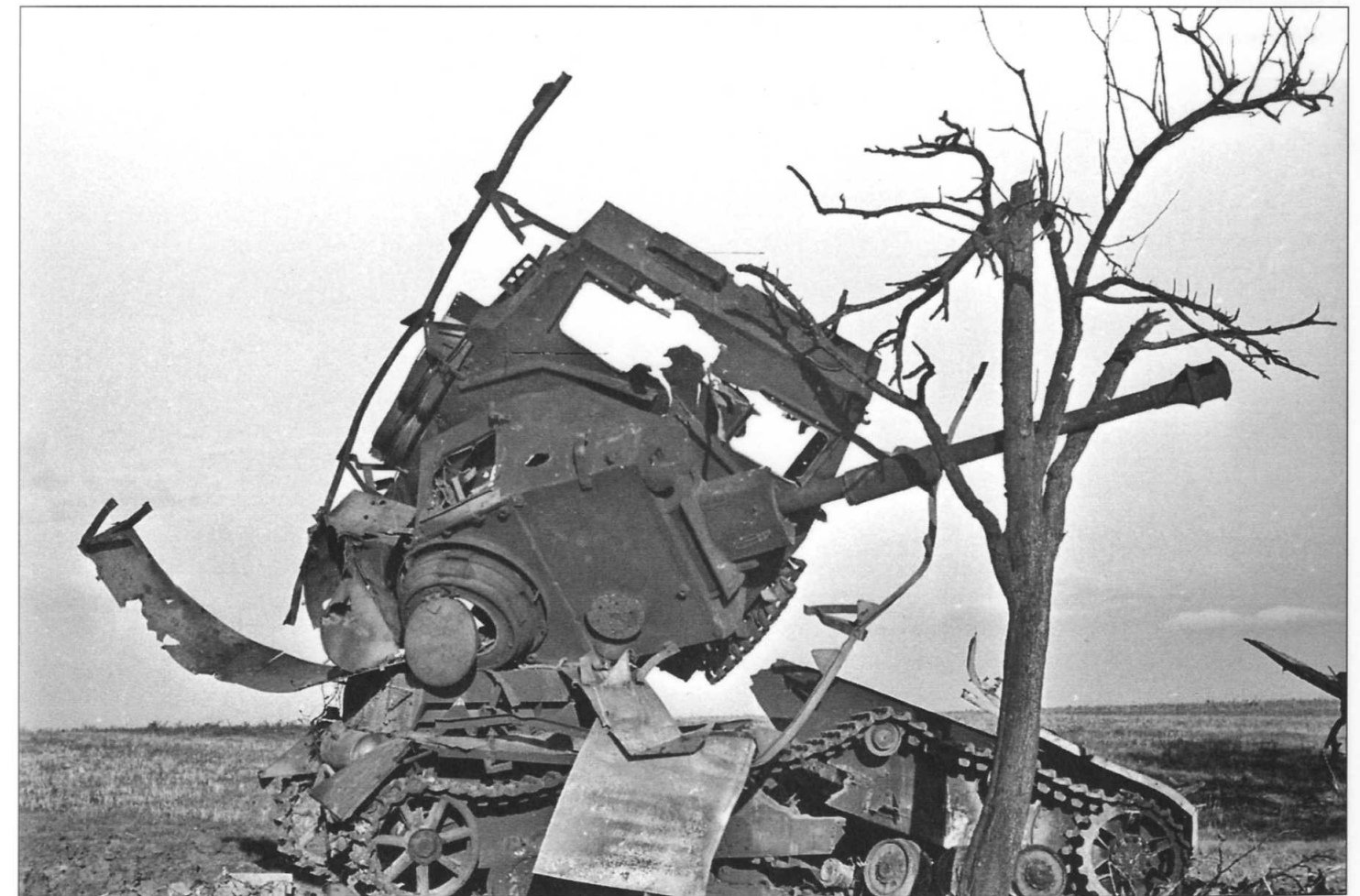
A completely destroyed PzKpfw IV stands twisted next to a charred tree. This Panzer has evidently suffered a violent explosion on board with its turret virtually blown off. Amazingly the vehicle's tracks are still intact.
