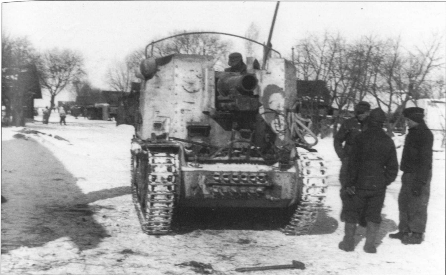
A 15cm schweres Infanteriegeschütz 33, which mounted the 15cm sIG33 infantry gun on a PzKpfw 38(t) chassis. 90 of these vehicles were built, serving with the sIG companies within Panzergrenadier regiments.
