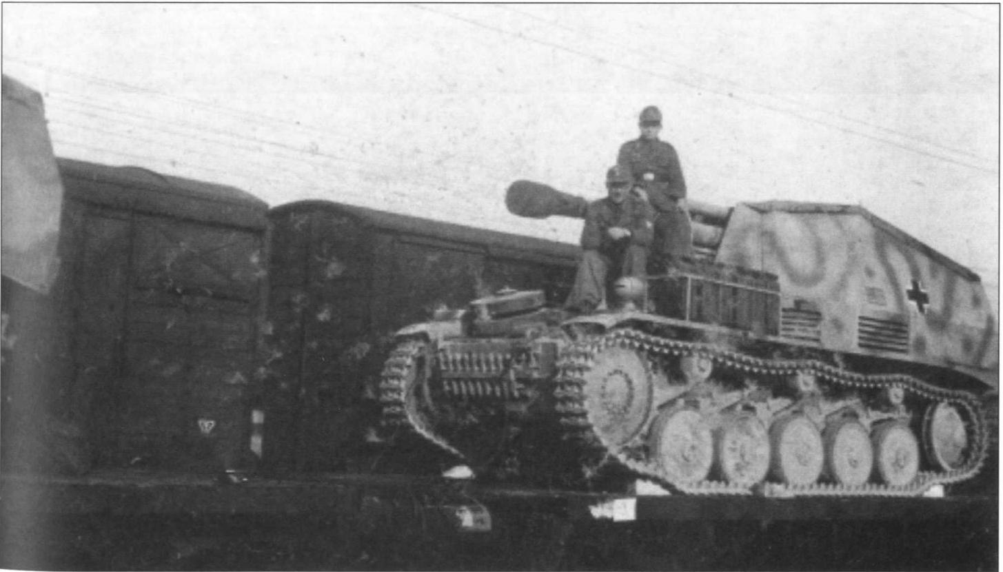
Two crewmembers can be seen sitting with their Wespe howitzer on board a flat bed railway car. Note the specially constructed rack to carry jerry cans of fuel for long road marches. This popular vehicle was armed with a 10.5cm leFH 18/2 L/28 gun and protected by a lightly armoured superstructure mounted on a chassis of a PzKpfw II. This vehicle served in armoured artillery battalions but was lightly armoured, and as a result many of them were lost in battle.
