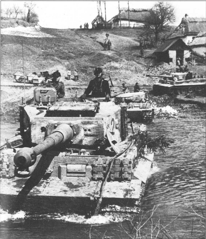
A Tiger tank carrying a full application of Zimmerit anti-magnetic mine paste wading across a river. This vehicle belongs to schwere Panzer Abteilung 506. In May 1943 schwere Panzer Abteilung 506 was formed and saw action alongside the 9th Panzer-Division. Within a year it had suffered heavily from continuous combat in Army Group North Ukraine.
