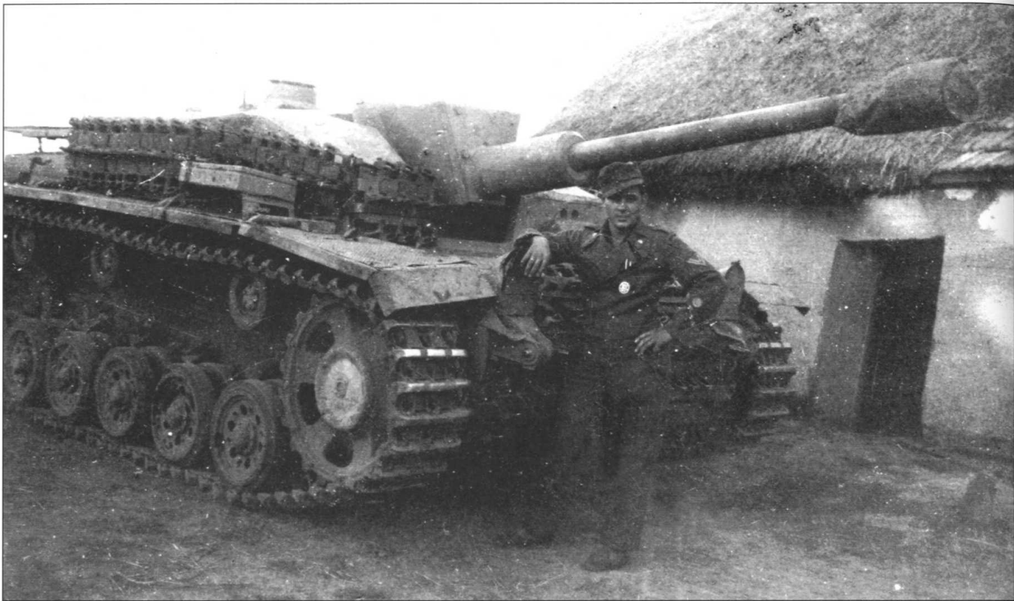
A crewman poses for the camera next to his StuG III Ausf F. Track links can be seen attached to the vehicle for additional armoured protection. Note the protective covering placed on the end of the 7.5cm gun's muzzle break to prevent dust particles and other foreign matter contaminating the gun tube.
