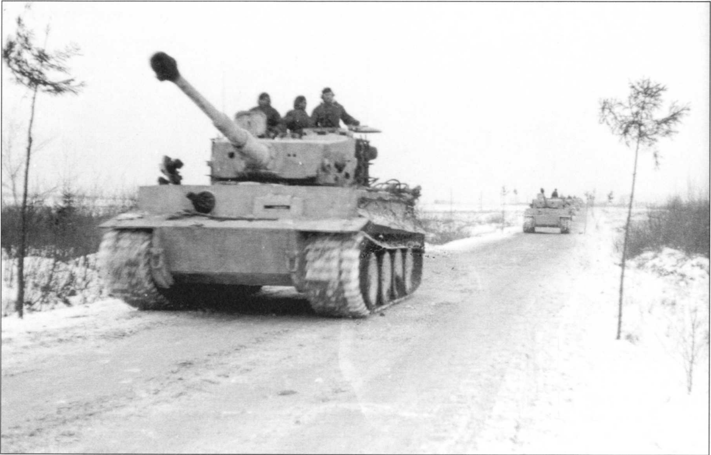
Two photographs showing Tiger tanks with an application of winter whitewash paint over a coating of Zimmerit anti-magnetic mine paste. By early 1944 the Tiger continued to play an important, mainly defensive, role.
