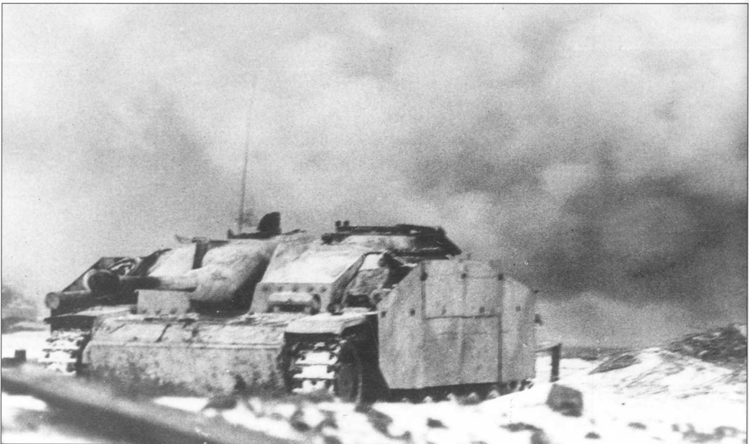
This photograph shows a StuG III Ausf G assault gun in the thick of battle. This vehicle is armed with a 7.5cm StuK 40 L/48 cannon, which both necessitated modification of the frontal superstructure and increased the overall weight to 21.3 tons.
