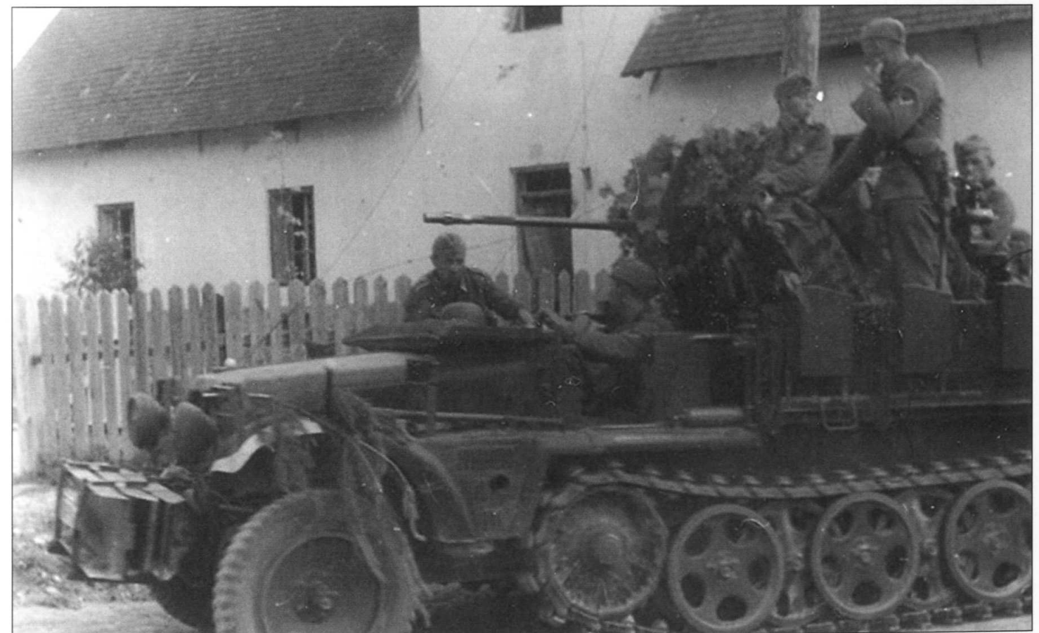
An SdKfz 10 advances through a destroyed village. This vehicle mounts a shielded 2cm Flak 30. Note the magazine containers on the drop sides. By 1944 both Wehrmacht and Waffen-SS mechanized formations were well-equipped with flak guns.
