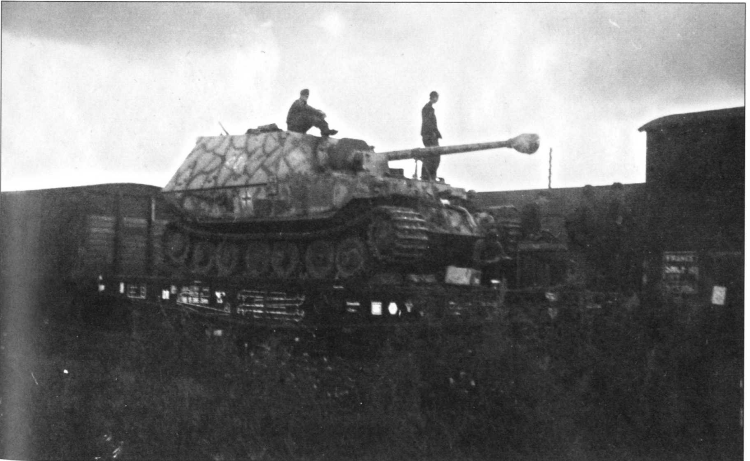
Two photographs showing Panzerjäger Tiger or Ferdinand Elefant tank destroyers that have been chocked and secured ready for their journey by rail. Due to their sheer size and weight, no more than six of these vehicles were permitted to be loaded on one train. These were interspersed with two flatcars to avoid overloading of the train, and also to prevent overloading of the bridges.
