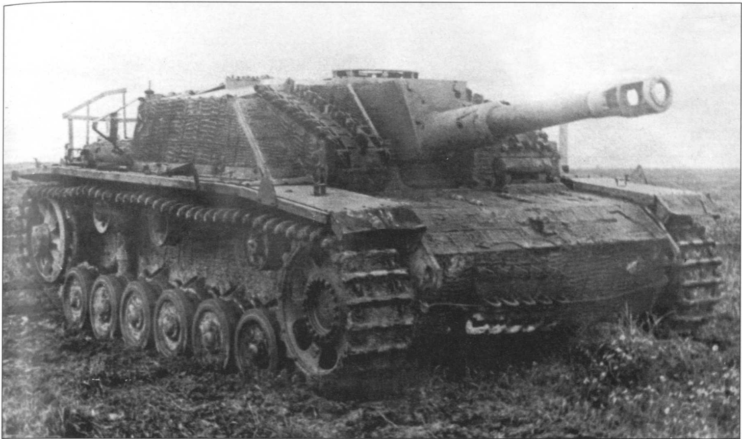
A 10.5cm Sturmhaubitze 42 displaying a very full coating of Zimmerit anti-magnetic mine paste. For additional armoured protection track links have been bolted to the vehicles glacis. The StuH 42 was used within StuG brigades to provide additional firepower both in attack and defence.
