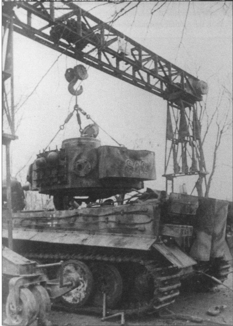
An interesting image showing one of the independent Tiger battalions undertaking mechanical work on a Tiger from SS schwere Panzer Abteilung 101 in 1943. The large portal crane is being used to remove the heavy turret for repairs.
