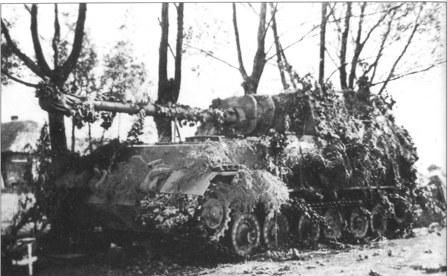
Here a well camouflaged Ferdinand Elephant has run out of fuel. This tank destroyer was capable of defeating all types of Soviet tanks, but the vehicle lacked cross-country mobility and was prone to breakdowns. Also, with no secondary armament they were vulnerable to infantry armed with magnetic mines and charges.
